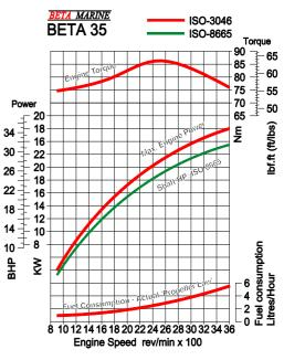
Fuel Consumption based on theoretical propeller loading - matched at full speed
